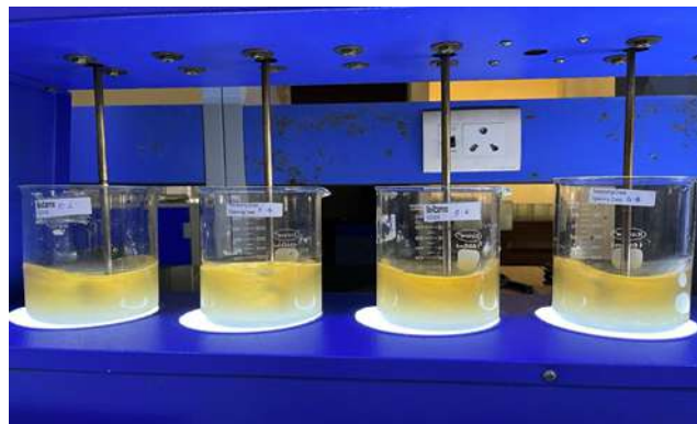
Fig 1: Jar test Apparatus to carry out coagulation-flocculation treatment on dye effluent
