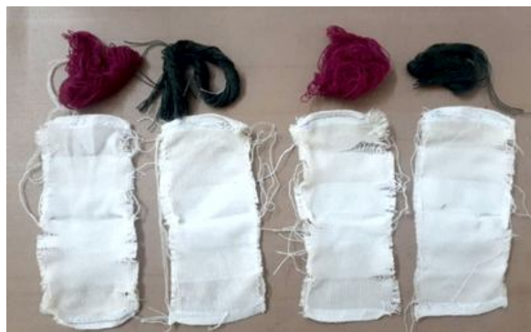
Figure 3 Exhaust dyed (left) and dope dyed (right) sample tested with (a) Method B, (b) Method C
