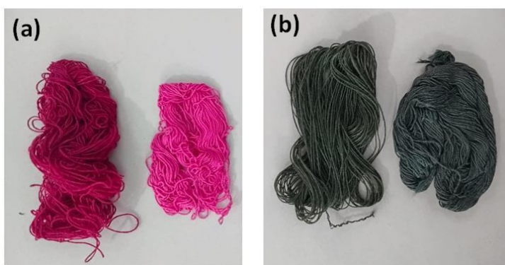
Figure 1 (a) Exhaust dyed sample, (b) Dope dyed sample before (left) and after (right) dye stripping test
